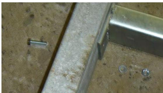
(bolt M8x30 RVS + spring washer M8 +nut M8)
